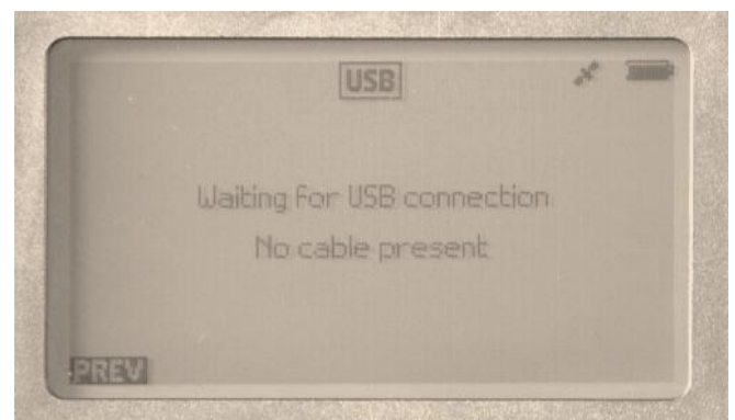
USB not active (Goniometer not physically connected to PC = cable issue)
