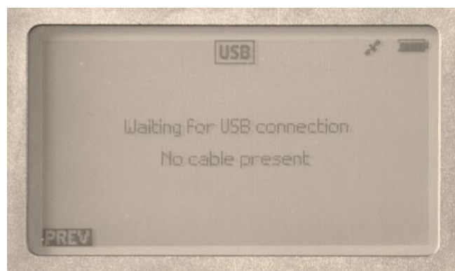
USB not active (Goniometer not physically connected to PC = cable issue)
